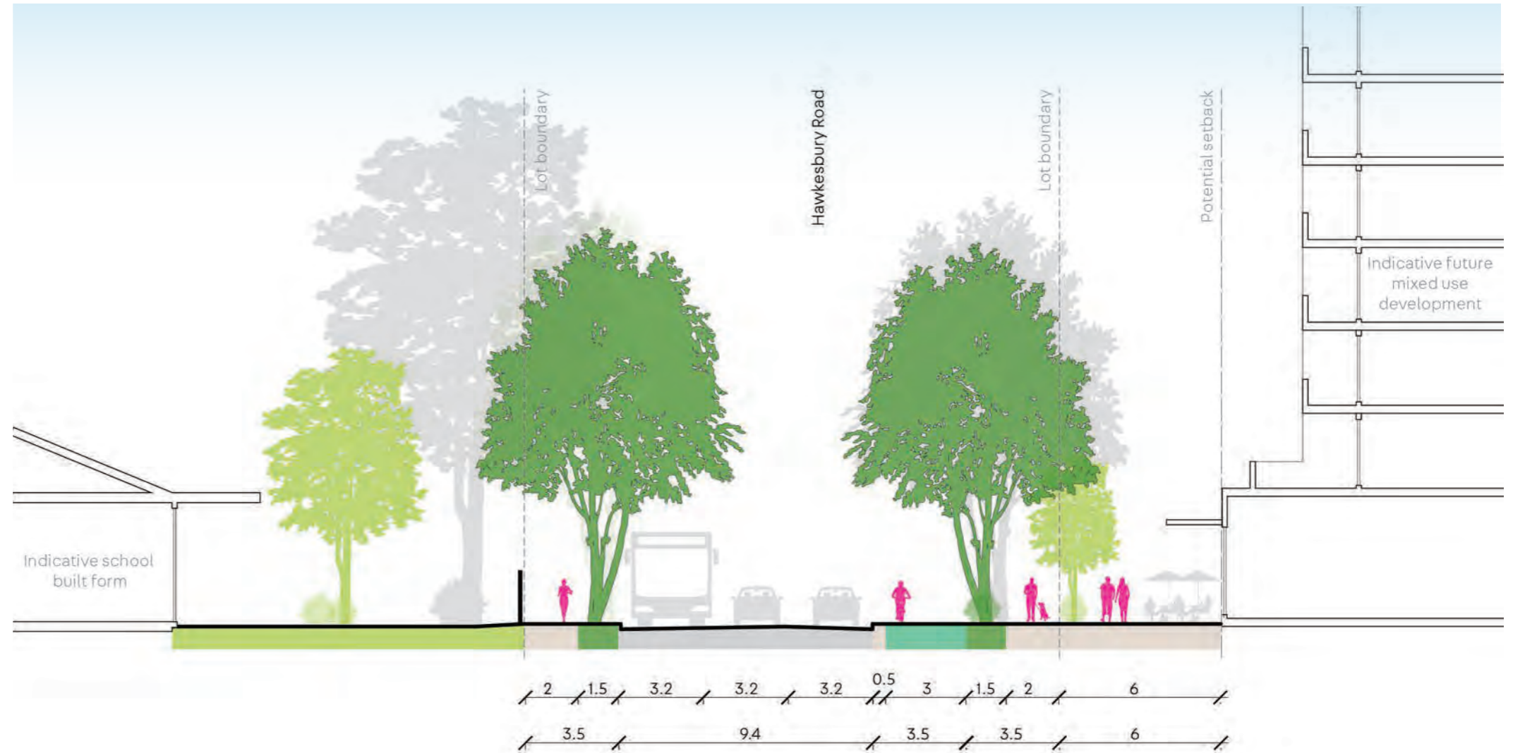
Section A through Hawkesbury Road near Westmead Public School - future condition
