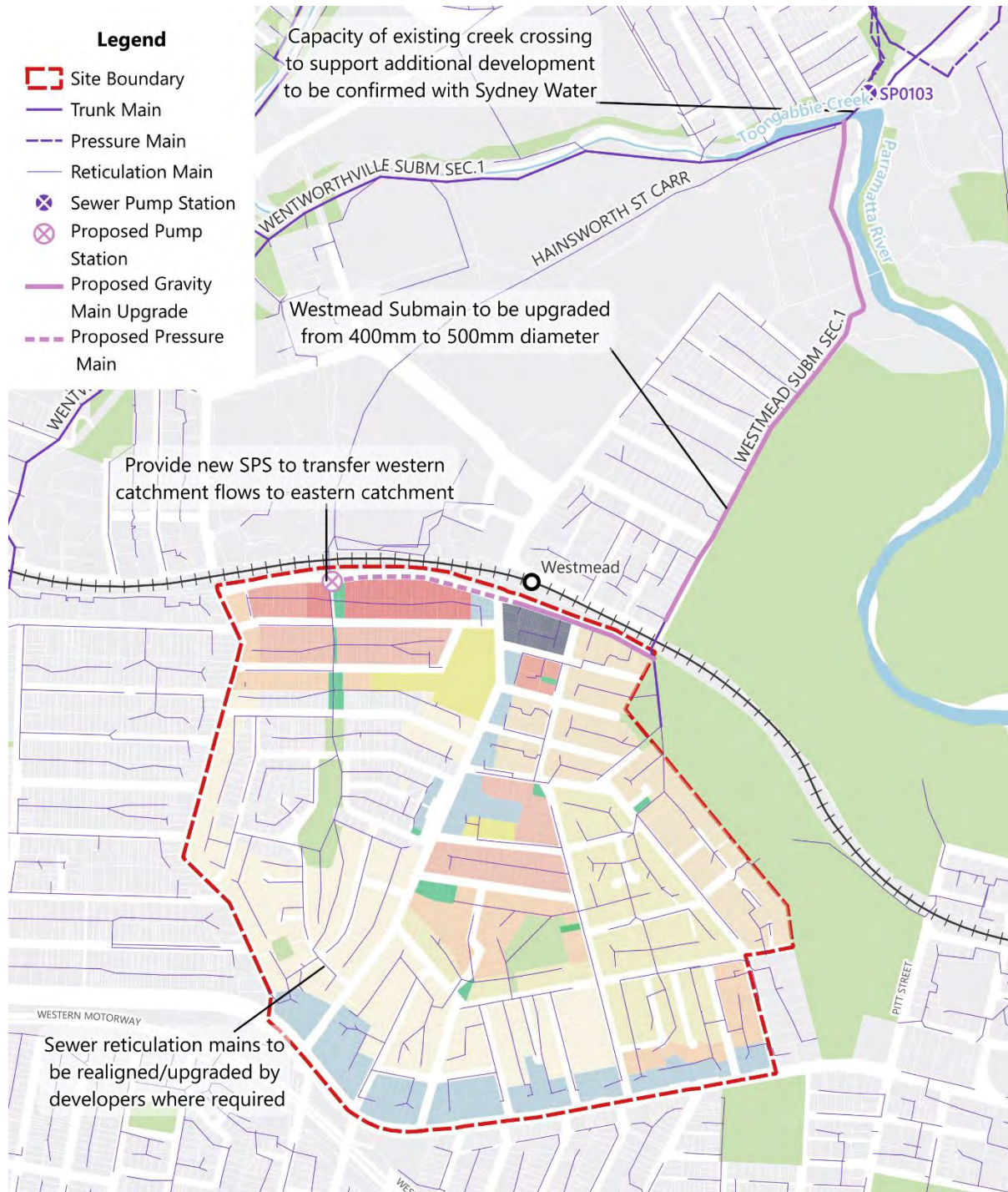
Figure 8 - Potential Sewer Servicing Strategy
