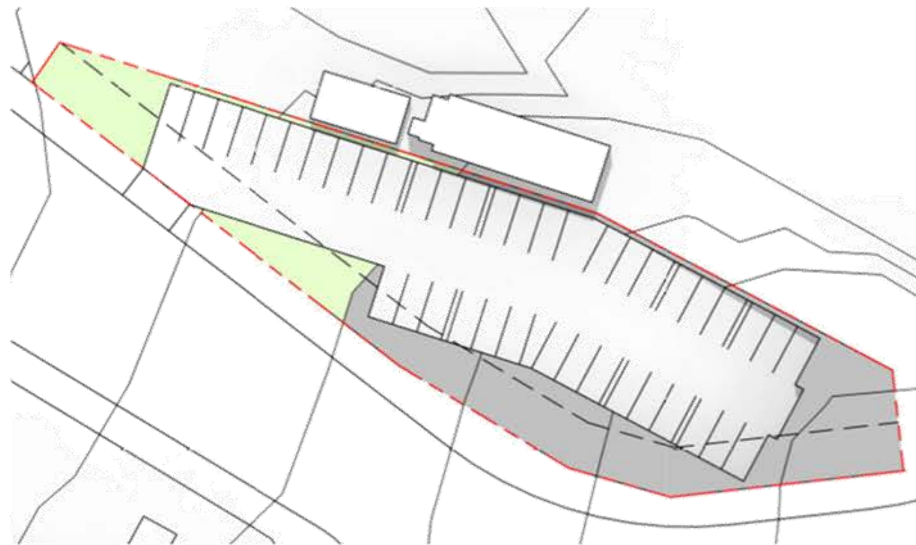
Indicative parking strategy for the site showing areas at-grade (surrounded by landscaping areas shown in green) and areas below ground (surrounded by earth shown in grey). The 5 metre front setback is shown by a black dashed line.
